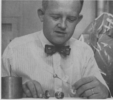
EARLY AND LATEST versions of krypton 85 cell are shown by Russell L. Maxwell (1332-4). Uncoated glass ball was previously placed within a metal container which functioned in the same manner as the carbon coatings do in the present model.
